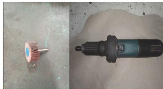
Gambar 9. *Grinding rotary*
